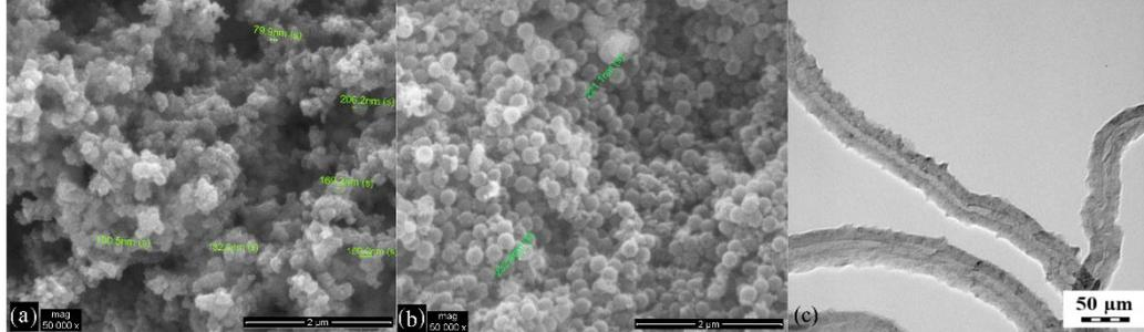
Figure 1: SEM images of TiC nanoparticles (a), CeMo nanocontainers (b); TEM image of carbon nanotubes (c).
