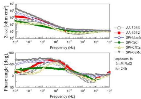
Figure 3: The Bode plots of the EIS spectra obtained for samples after 24 hours of exposure to corrosive environment.
