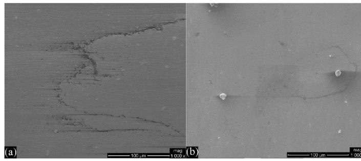
Figure 2: SEM images of the cross-section of SW-CNTs and SW-TiC at the welded nugget.
